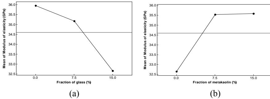
**Figure 7 :** Main effect plot for modulus of elasticity, (a) particle size of glass, (b) fraction of glass, (c) fraction of MK.
