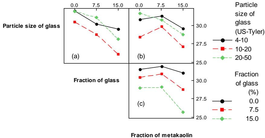
**Figure 6 :** Interaction effect plot for compressive strength, particle size and fraction of RG and fraction of MK
