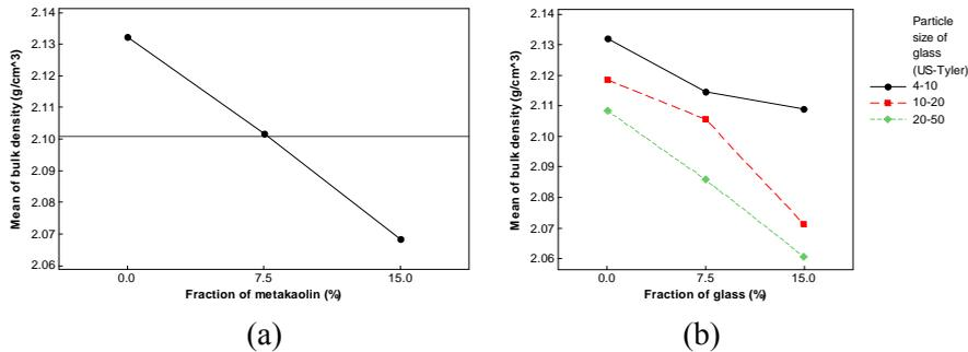
**Figure 3 :** Main effect plot (a) and interaction effect plot (b) for bulk density
