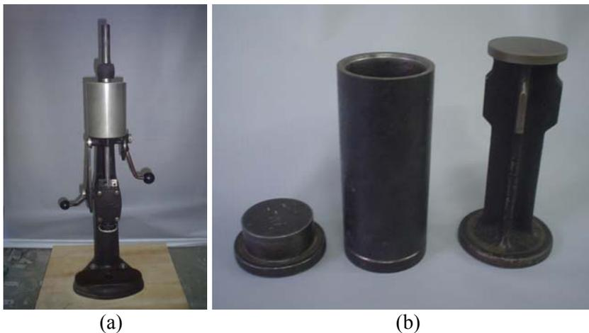
**Figure 1 :** (a) hammer (b) metallic moulds
