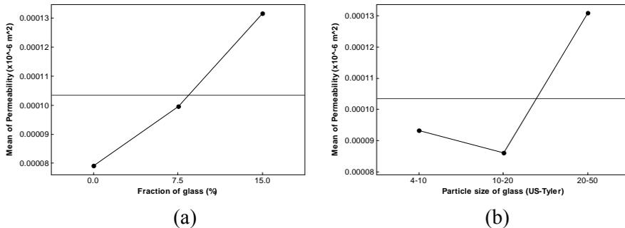
**Figure 5 :** Main effect plot for oxygen permeability; (a) fraction of RG; (b) particle size of RG
