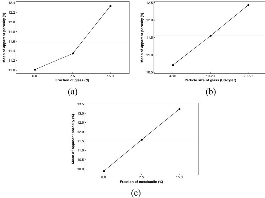
**Figure 4 :** Main effect plot for apparent porosity, (a) fraction of RG, (b) particle size of RG, (c) fraction of MK
