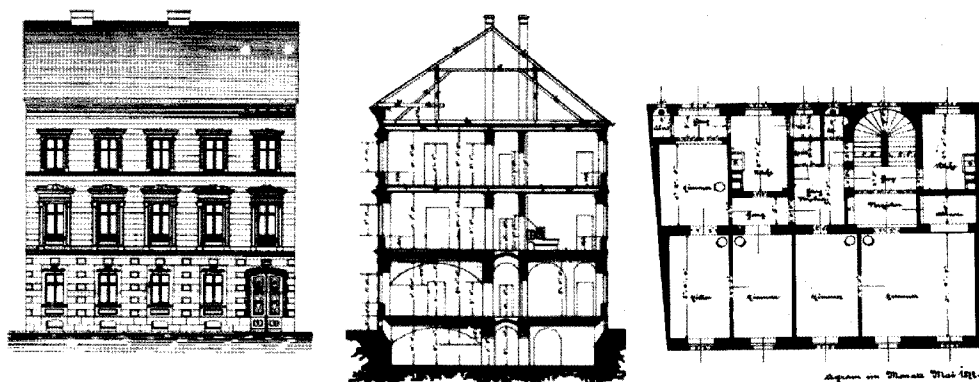
Figure 2 : Typical built-in apartment house from period up to 1940: street façade, section and 1 st floor plan.
