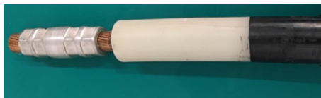
Figure 8: Image of the cable joint
