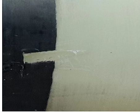
Figure 2: Irregularities in semi-conductive stripping
