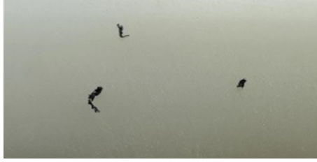
Figure 5: Stains on the main insulation
