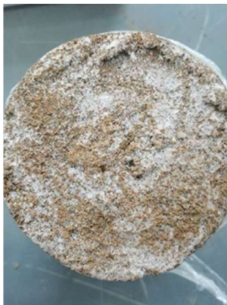
(a) Ice crystals on the surface of frost heave soil samples
