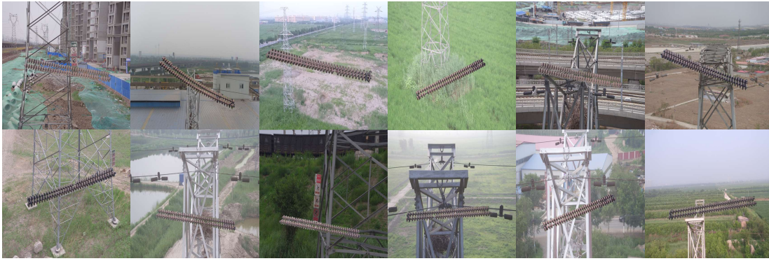
b. Image of damaged insulator
