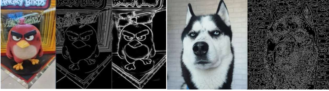
Figure 2: Experimental result of edge detection using Canny operator
