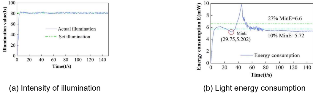
Figure 8: Energy consumption traversal and energy consumption optimization at 81 lx
