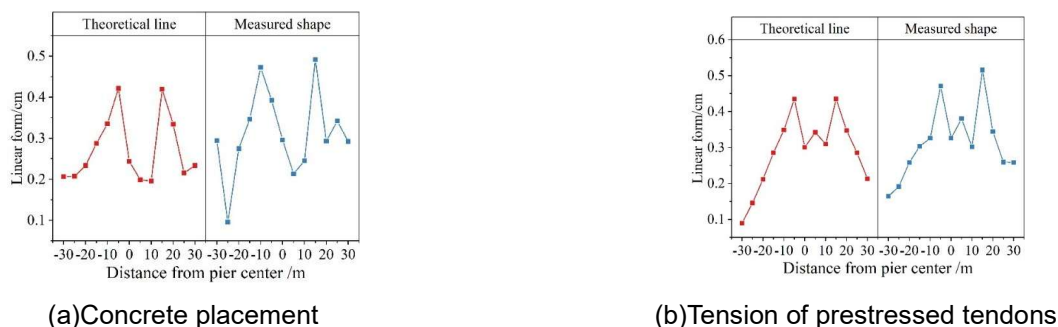
Figure 4: Comparison of line shape of 4# pier 6# beam section during construction
