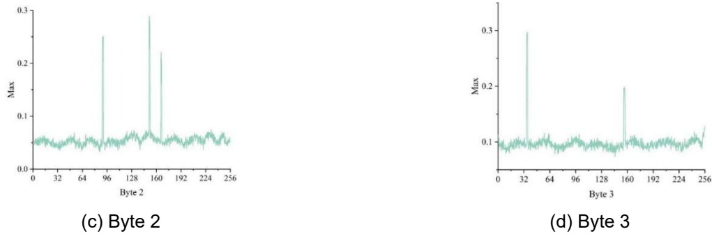
Figure 6: The peak absolute distribution of the correlation coefficient curve of the DPA attack
